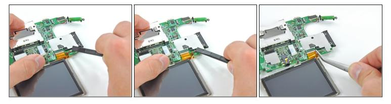
Use the flat end of a spudger or your fingernail to flip up the retaining flap on the lower LCD power ribbon cable ZIF socket.
