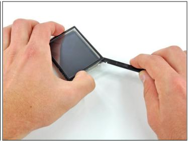
• Repeat the above procedure for the remaining two corners to pry the touchscreen off the LCD frame.
