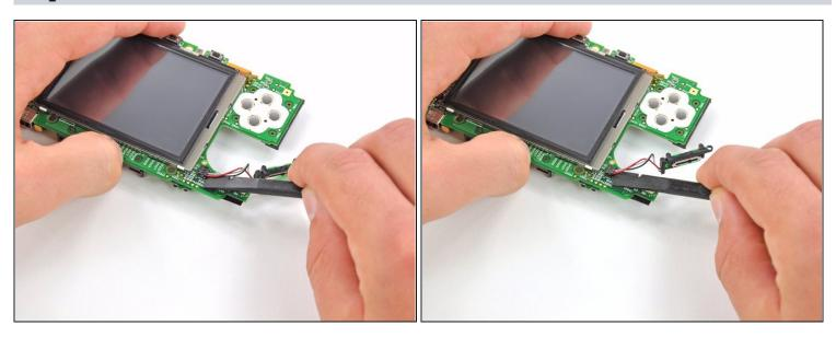
• Use the flat end of a spudger to pry the volume switch connector out of its socket on the motherboard.
