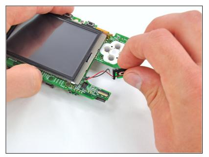
• Remove the volume switch from the motherboard.
