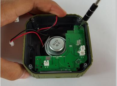
• Use Phillips PH00 screwdriver to remove the three screws holding the motherboard in place.
