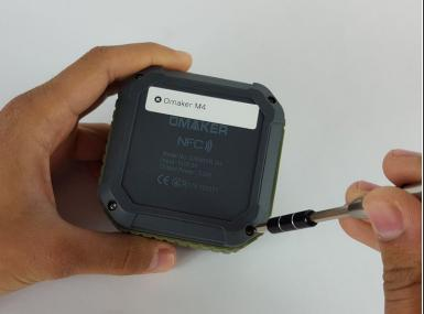
Use a T6 Torx screwdriver to remove the four 9mm screws from the back of the device.
