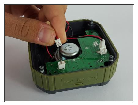
Remove the speaker wire by carefully pulling the plug out of the socket on the motherboard.
