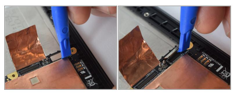
Using a plastic opening tool, unplug the ribbon cable indicated in the picture.
