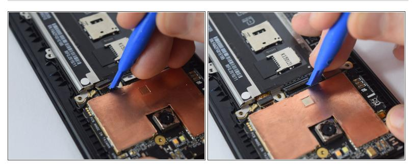
Using the plastic opening tool, disconnect the ribbon cables from their connectors by gently prying them up.
