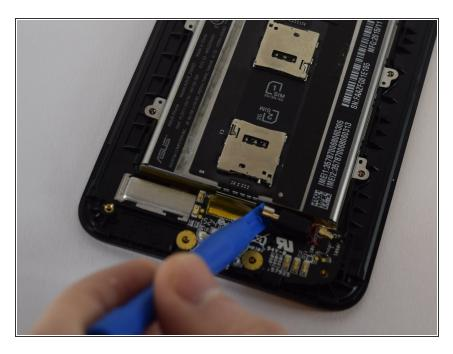
Using a plastic opening tool, gently pry the vibration motor from its mount.
