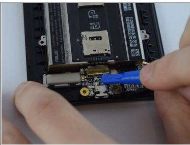
Using the plastic opening tool, unlock the ribbon cable attaching the battery to the circuit board by prying up the yellow tab.
