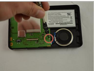
Use your T5 Torx screwdriver and unscrew the two 5.0 mm screws on the motherboard.
