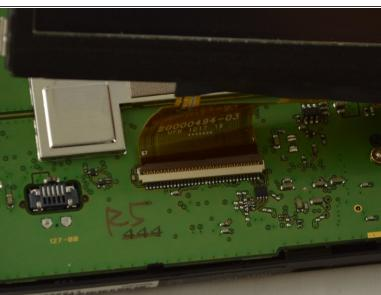
Remove the piece of tape that is covering the connecting point of the motherboard and display.
