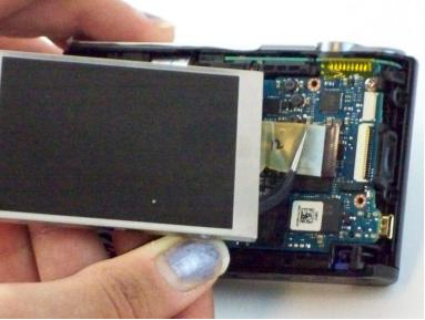
Gently pull on the ribbon wire disconnecting from the ZIF connector (connecting the LCD screen to the motherboard) with the tweezers.
