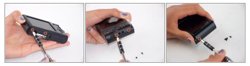
Remove the five 4.0 mm Phillips #000 screws on the back panel.
