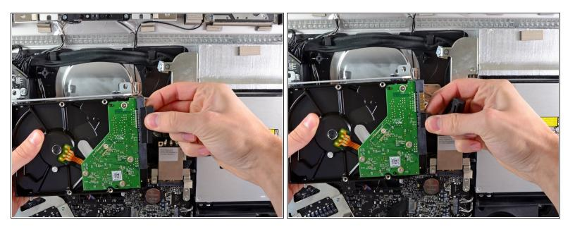
Disconnect the SATA data cable and SATA power connector from their respective sockets by pulling each connector away from the hard drive.
