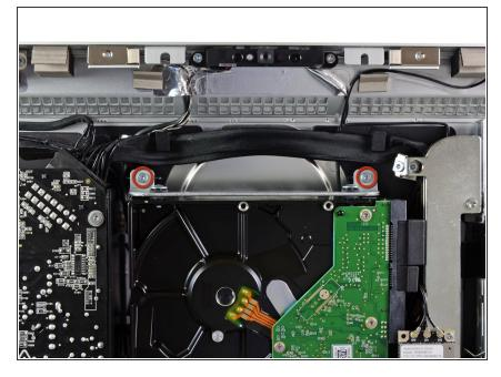
Remove the two 9 mm T10 Torx screws securing the upper hard drive bracket to the outer case.
