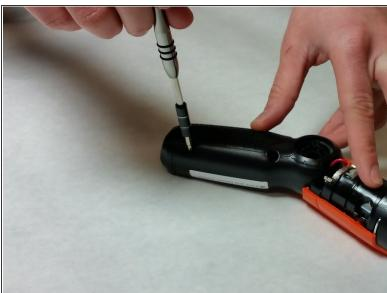
Remove the four 15mm Phillips #1 screws.
