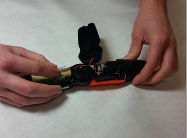
Use a plastic opening tool to pry the casing apart.
