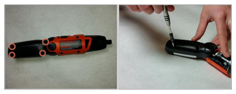
• Remove the four 15mm Phillips #1 screws.
