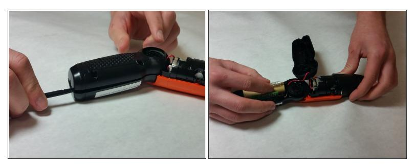
• Use a plastic opening tool to pry the casing apart.
