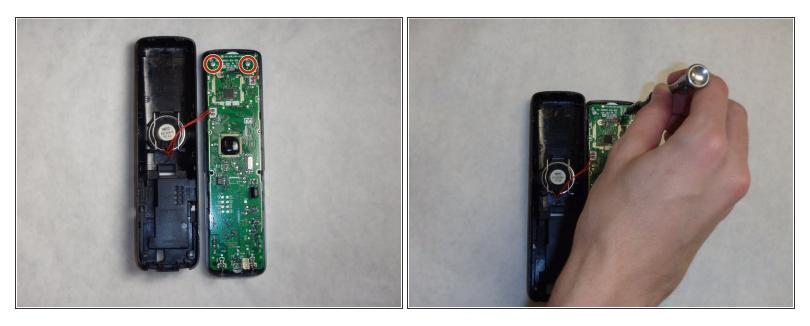
• Remove the two 9mm screws located inside the back cover at the top.
