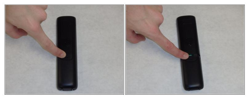
• Push down on the battery cover in the direction of the arrow located on the back of the phone.
