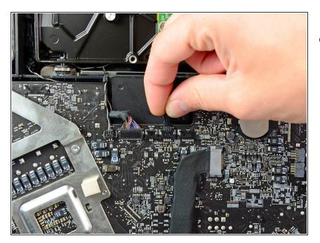
Pull the hard drive fan connector toward the top edge of the iMac to disconnect it from its socket on the logic board.
