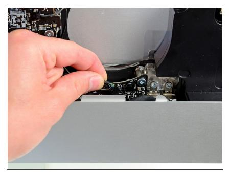
• Pull the SD board cable out of its socket on the logic board.
