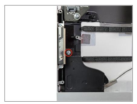
Remove the single 13 mm T10 Torx screw securing the left speaker to the outer case.
