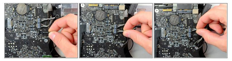
Disconnect the microphone, left speaker, and right speaker cables by pulling their connectors toward the right side of the iMac.
