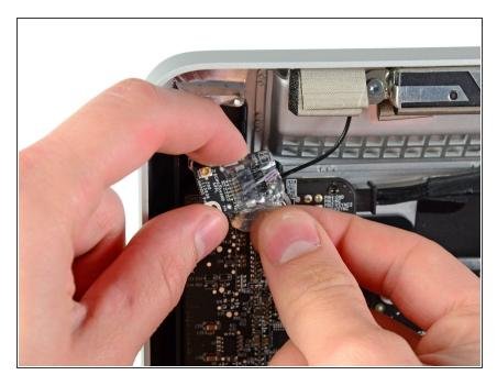
Remove the piece of tape wrapped around the Bluetooth board.
