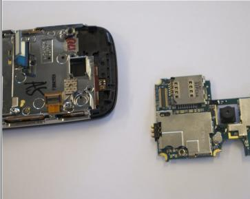
The circuit board will still be held on by a blue and black ribbon. Remove the entire circuit board by gently tugging the ribbon upwards.
