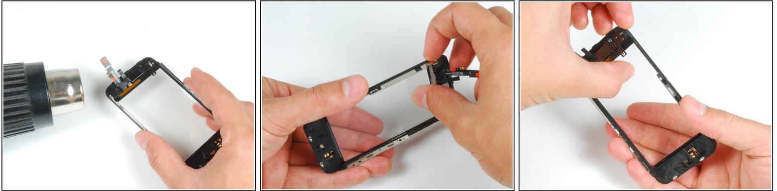
**⚠** Be careful when using a heat gun in the forthcoming steps. Use it at a very low heat setting, and make sure not to melt the touch screen plastics or Home button. The metal frame tends to conduct heat very well so try to avoid touching these hot areas.
