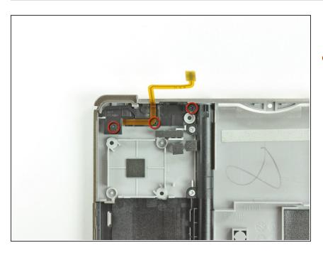
Remove the three 3.6 mm Phillips screws from the button housing.
