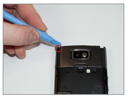
Using an iPod opening tool, remove the screw cover in the top left corner by lifting it up.
