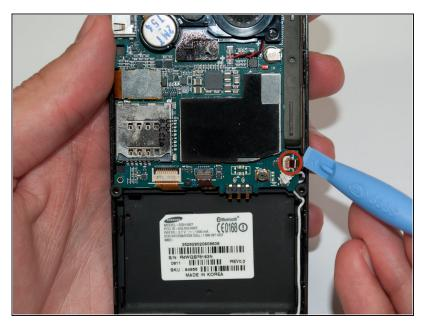
Using iPod opener tool, unlatch and remove the front panel ribbon cable at bottom right of motherboard.
