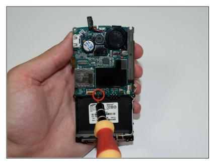
Using a Phillips #00 screwdriver, remove the 3.5 mm screw at the bottom center of motherboard.
