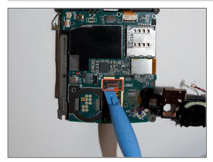
Using iPod opener tool, unlatch and remove the camera ribbon cable.
