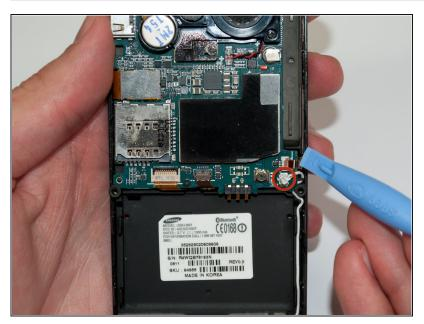
Using the iPod opener tool, remove the microphone cable at bottom right of motherboard.
