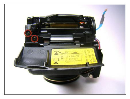
Remove the two Phillips screws located underneath the CF card cover.
