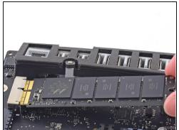
• Slightly lift the rightmost side of the SSD and firmly slide it straight out of its socket on the logic board.
