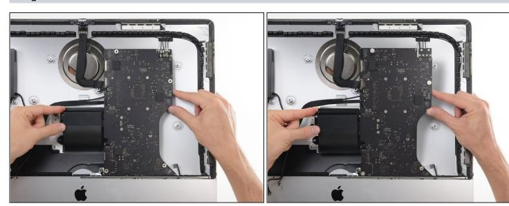
• Tilt the top of the logic board away from the rear enclosure.
