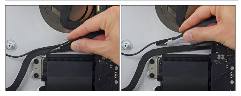
• Peel up the piece of tape connecting the left speaker connector to the SATA power and data cables.
