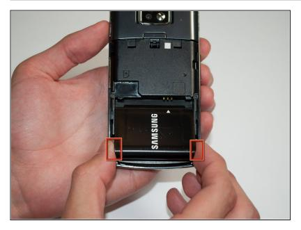
Grasp the bottom corners of the battery with two fingers and gently lift.
