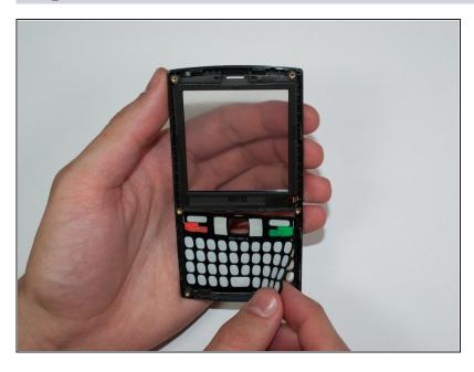
Grasp the rubber keyboard in the corner with your fingers and lift to remove.
