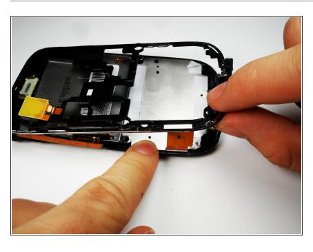
Remove the metal frame. Slip out the copper clips still attached to the bottom frame from the frame carefully.
