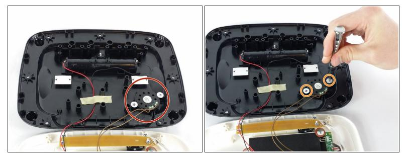
(i) The speaker should be located at the bottom-right side of the back cover from your perspective.
