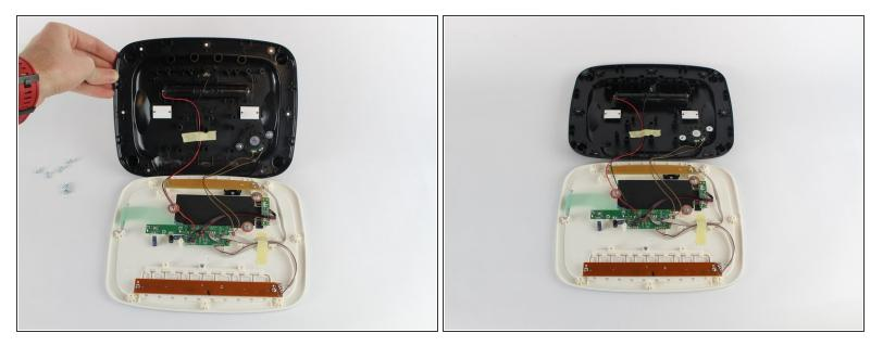
Gently remove the back cover then flip it 180 degrees so that the back cover of the device is now face-down.
