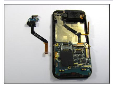
• Peel the Input jack assembly out of the case.
