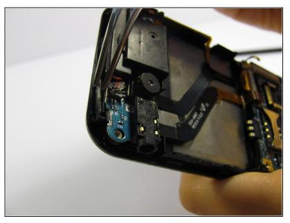
• Peel the button sensor off the top of the case.
