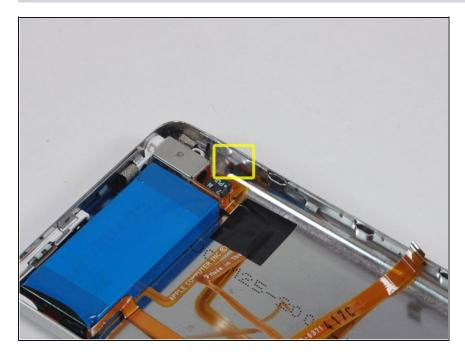
Now to repair the damage caused by liberating the internal parts of the iPod Classic! It is highly likely that at least one of the metal clips in the lower case has been bent upward. These clips must all be pointing downward in order to reinstall the rear panel.
