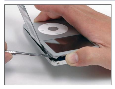
• Continue to push up on the front panel with the metal spudger until the metal clip releases.
