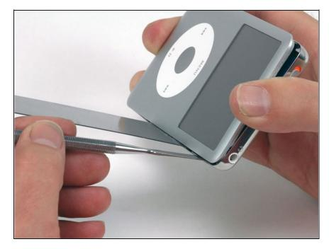
• Gently wiggle the metal spudger down so that it is all the way in the rear panel.
