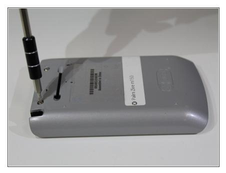
Use T6 bit of screwdriver provided in the iFixit toolkit. Unscrew the two screws at the top of the device.
