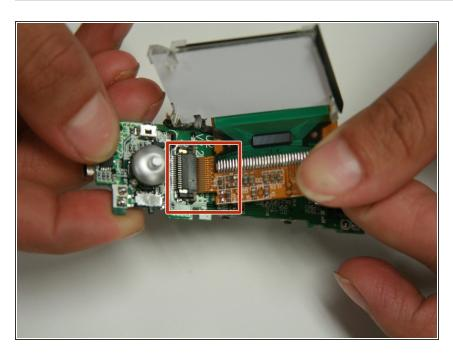
Slide the display screen chip out of the motherboard. Insert a new display screen.
