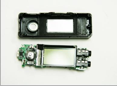
Using the plastic opening tool from the iFixit toolkit you will be able to wedge in between the device case and the motherboard. Push down on the exposed end of the device and the motherboard should pop up.
