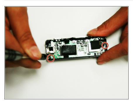
Using the PH000 drill bit from the iFixit toolkit, unscrew the 2 screws that detach the motherboard from the device.
