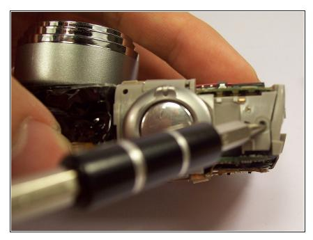
Remove the screw next to the shutter with a Philip's head screw driver.
