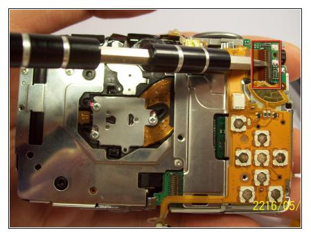
Remove the orange ribbon cable by lifting the ZIF connector attached to the ribbon with a flat head screw driver or spudger.
