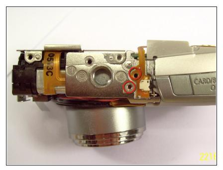
Remove the two screws near the the tri-pod mount with a Philips head screw driver.
