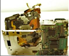
With the motherboard casing detached, remove the short orange ribbon by lifting the ZIF
