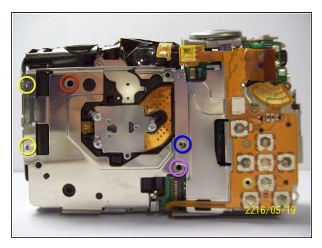
Once the LCD and Backlight are detached, remove the larger screw marked in red in the picture as well as the four smaller sized screws marked in blue.
