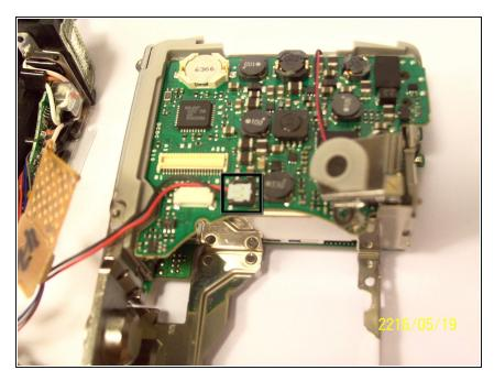
Remove the last wires connected to the motherboard. You can remove it by gently lifting it upwards.
