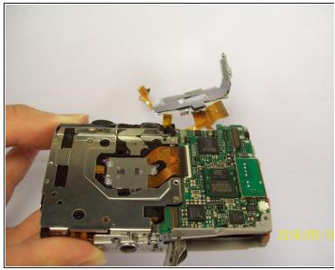
Carefully lift the shutter along with the ribbon connected to it. This will remove the casing around the motherboard.
