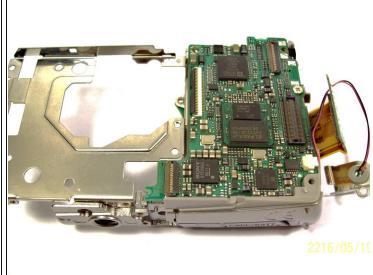
Place a flathead screwdriver and gently lift the circuit attached, as shown on the picture.
