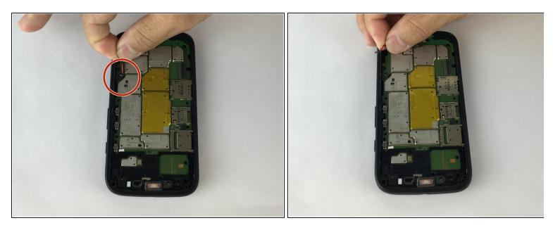
• Gently lift up the battery cable connector, it should come out very easy.
