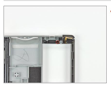
Remove the 3.6 mm Phillips screw from the right shoulder button cover.
