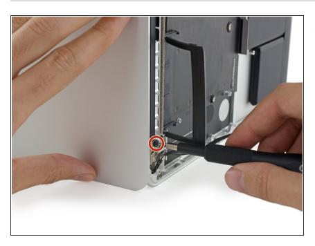
While holding the display and upper case together with your left hand, remove the remaining T8 Torx screw from the lower (closer to the table) display bracket.
