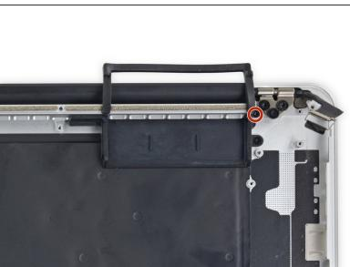
• Remove the two 3.2 mm T5 Torx screws securing the aluminum hinge covers to the upper case.
