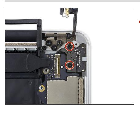
Remove the two 4.0 mm T5 Torx screws from the MagSafe 2 board.
