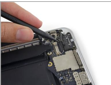
Use the tip of a spudger to flip up the display data cable lock and rotate it toward the MagSafe 2 power port side of the computer.
