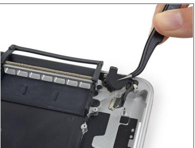
Remove the two rubber hinge covers.
