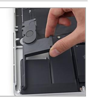
Remove the right speaker by pulling it slightly away from the side of the upper case, and out from under the aluminum tab blocking it in.
