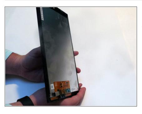
Remove the screen and digitizer from the case completely. To reassemble your device, follow these instructions in reverse order.
