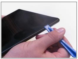
Avoid prying near bottom right hand side due to LCD Connector
