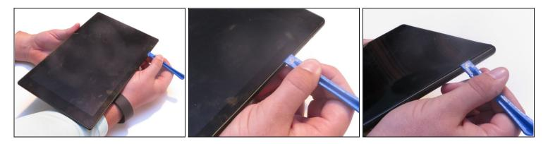
⚠ Avoid prying near bottom right hand side due to LCD Connector
