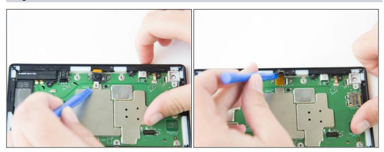
Detach the connector using a plastic opening tool or spudger.
