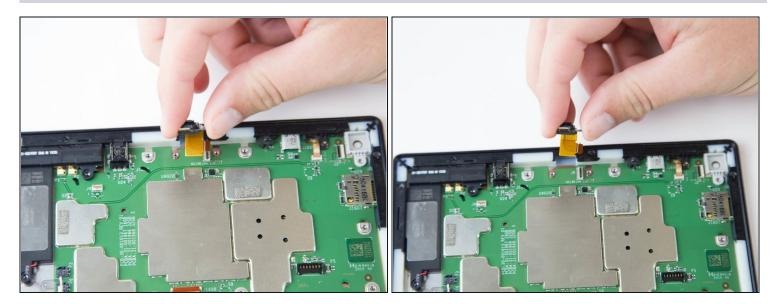
• Grip the camera and lift up to detach the ZIF connector from the motherboard.
