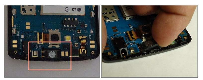
Use a plastic opening tool or your finger to carefully disconnect the speaker.
