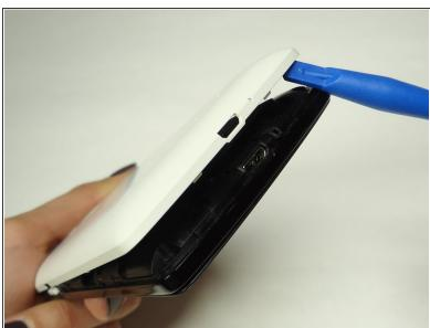
Use the plastic opening tool to pry off the back cover.
