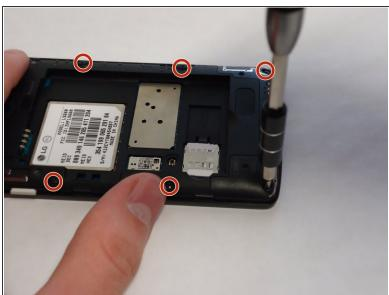
Remove eight 4mm screws using a Phillips head 000 screwdriver (PH000).
