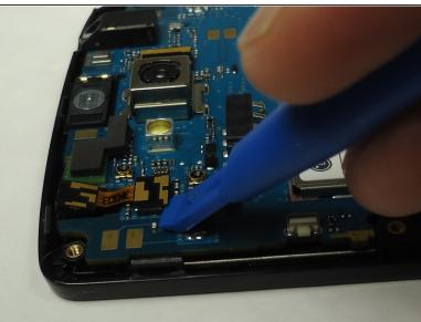
• Use the plastic opening tool to carefully pry the front-facing camera from the motherboard.
