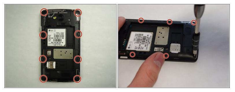
• Remove eight 4mm screws using a Phillips head 000 screwdriver (PH000).
