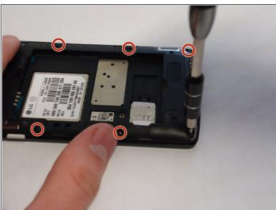
Remove eight 4mm screws using a Phillips head 000 screwdriver (PH000).
