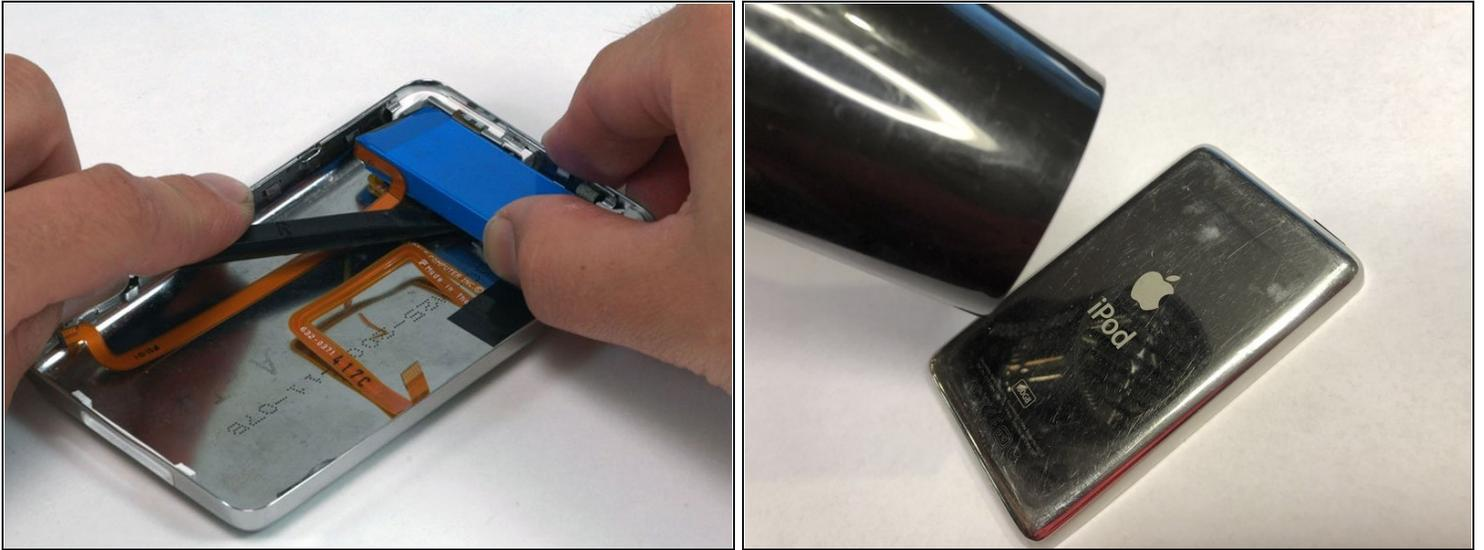
**⚠** The battery is attached to the rear panel with adhesive. Be careful not to tear the orange headphone jack or hold button ribbon cables when removing the battery.
