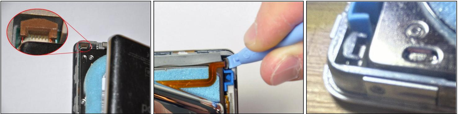
⚠ **The lock tab securing the battery flex cable is very delicate.** Pulling too much or pulling the white part of the connector easily risks pulling it completely off the main board. Once it's ripped off of the main board, repair of the battery connector will be very difficult.
