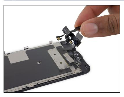
Remove the front-facing camera and sensor cable.
