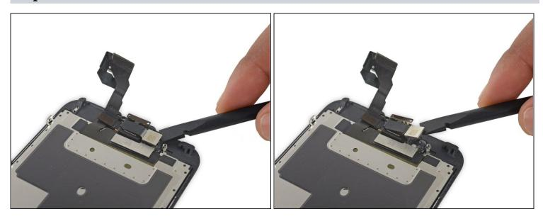
Use the flat end of a spudger to nudge the front-facing camera from its housing.
