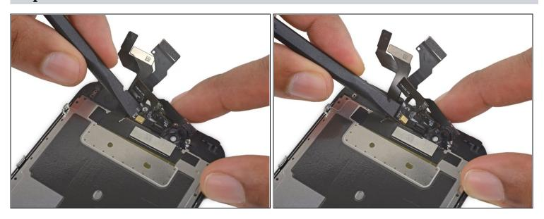
• Use the flat end of a spudger to gently break up the adhesive securing the microphone to the front panel.
