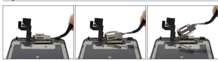
Lift up and remove the earpiece speaker bracket, peeling up the bracket gasket as you go.
