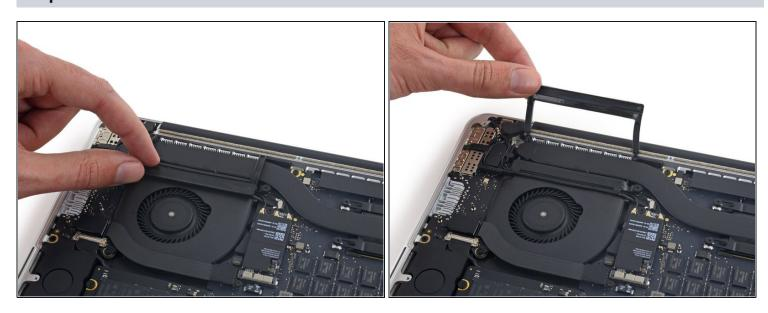
Peel the rubber cover up off the right fan and fold it out of the way.
