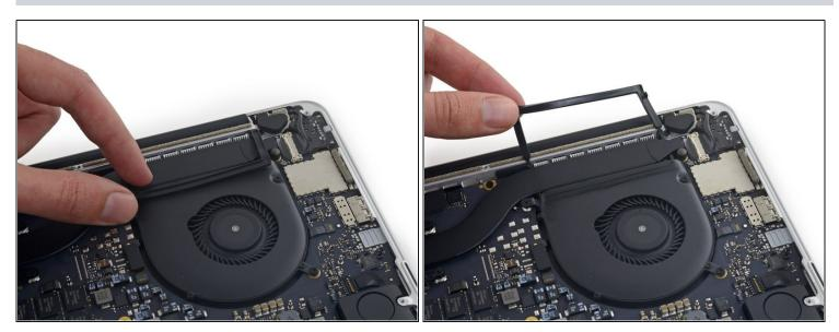
Peel the rubber cover up off the left fan and fold it out of the way.
