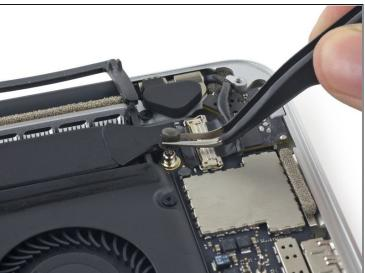
Remove the small rubber cap from the screw at the end of the heat sink.
