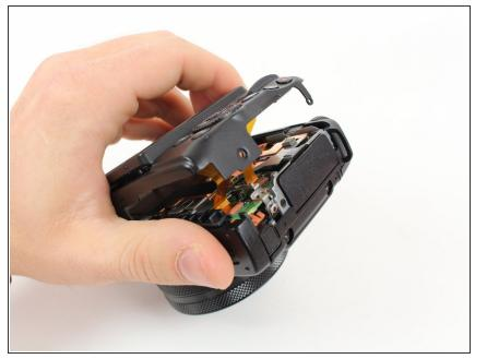
• Lift the back casing up far enough to expose the ribbon cables.
