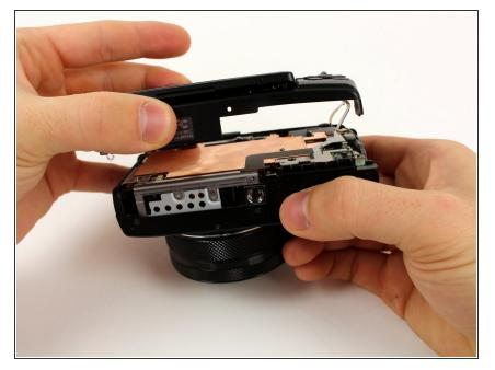
• Carefully lift the back casing away from the camera.
