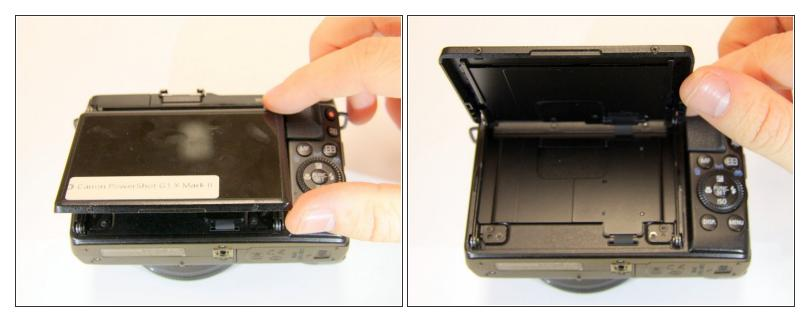
• Rotate the LCD screen away from the camera.
