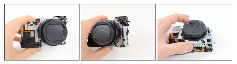
A Lay the camera on a flat surface while performing these steps because removing the frame causes the camera to fall apart.
