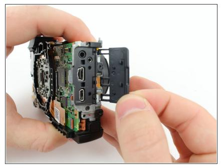
Remove the rubber dust cover from the camera by moving the hooks away from the three prongs holding them in place and then pulling the cover away from the camera.
