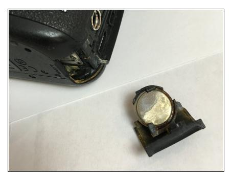
Replace battery and reassemble.
