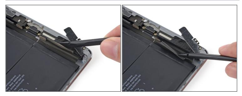
• Use the flat end of a spudger to fold the wide left-hand piece of tape away from the left speaker.
