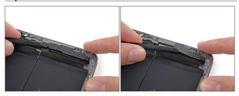
• Use the flat end of a spudger to loosen the foam adhesive securing the Wi-Fi antenna to the left speaker.
