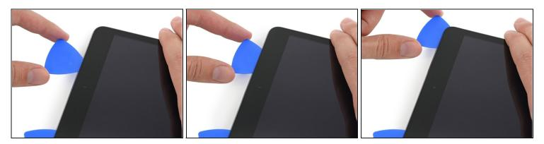
• Insert the previous pick deeper into the iPad and slide it away from the camera toward the corner.
