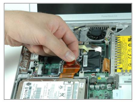
Use the orange plastic loop to disconnect the hard drive cable from the logic board.
