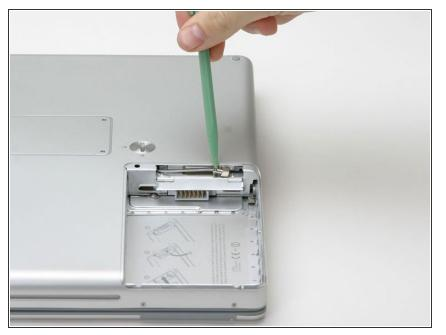
Use a spudger or flathead screwdriver to disconnect the Airport antenna from the card.
