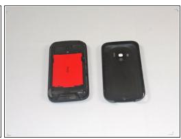
Remove back cover by applying pressure and sliding up towards the top of the phone.
