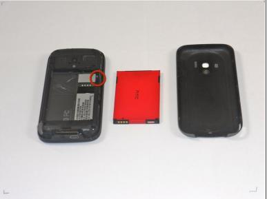
Remove the battery by lifting from slot on the right hand side.
