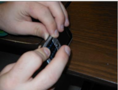
Snap the front case back in place with the bottom case with your fingers
