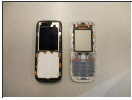
♠ Separate the front case from the back case using the iPod opener
