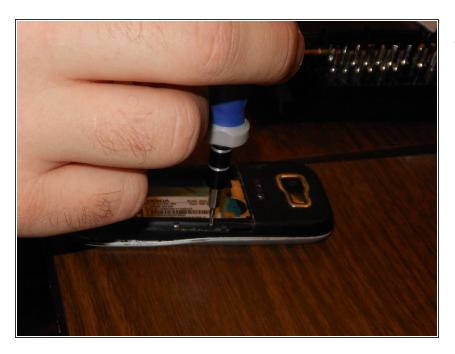
Reassemble screws with microscrewdriver
