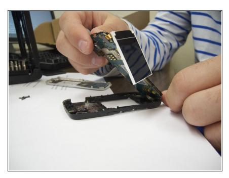
Carefully remove the computer chip and screen out of the black case with your fingers
