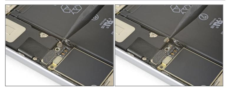
• Use the point of a spudger to pry up and disconnect the antenna cable from the bottom of the logic board.
