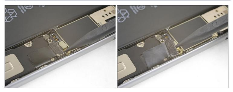
• Use the point of a spudger to pry up and disconnect the Lightning connector cable from the logic board.
