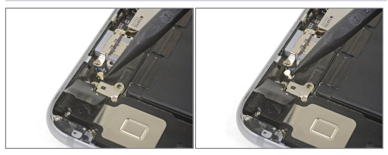
• Use the point of a spudger to pry up and disconnect the antenna cable from the Lightning connector assembly.
