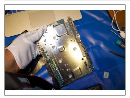
Remove the single 2.4 mm screw located on the metal casing at the top of the motherboard.
