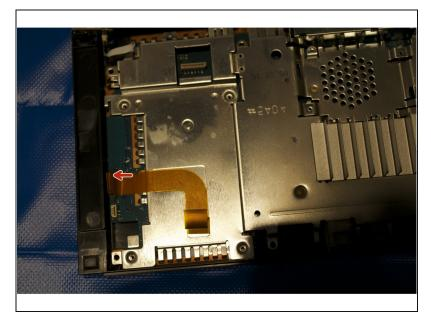
There is a ribbon attached to the motherboard here. With your spudger, gently detach the ribbon from the motherboard's connection.
