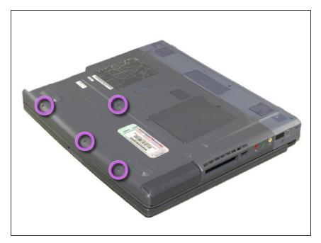
Remove the four 16 mm screws bordering the edge of the laptop using a Phillips #0 screwdriver.
