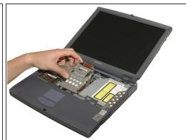
Remove the four 4mm Phillips screws around the hard drive.
