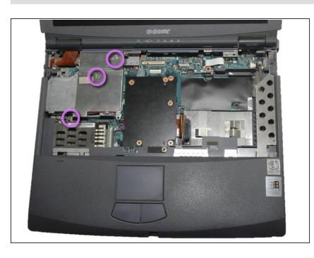
Remove the three 6mm brass colored, Phillips screws that hold the fan cage in place.
