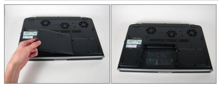
• Pull up on the battery to remove it.
